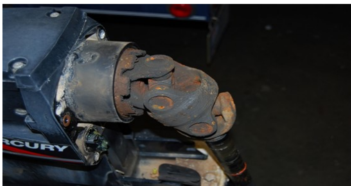
Driveshaft bellows failure has caused corrosion damage to this u-joint assembly, and certainly to the gimbal bearing that supports the driveshaft inside the housing where the bellows mounts. Photo: Pete Stevenson
