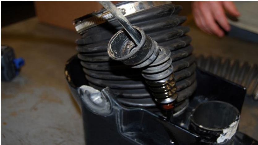
Failed shift cable bellows. Note the broken bellhousing casting.
