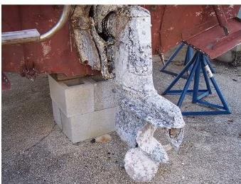
This lower unit became a huge anode to other more noble metals connected by seawater, sacrificing much of its aluminum metal. (courtesy Boat-US)
