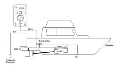
Reference electrode setup for measuring corrosion potential (courtesy of Reliability Direct, Inc.).
