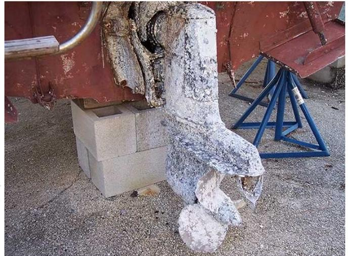
This lower unit became a huge anode to other more noble metals connected by seawater, sacrificing much of its aluminum metal. (courtesy Boat-US)
