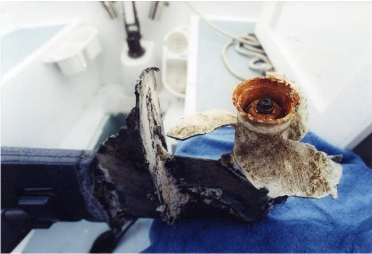
Nearby boats with steel alloys overwhelmed the anode on this kicker and destroyed the lower unit while docked. (courtesy Boat-US)
