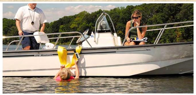
Commercial slings are available to assist in recovery. However, they should be tested to make sure that they will work with your particular boat. (courtesy BoatUS Foundation)
