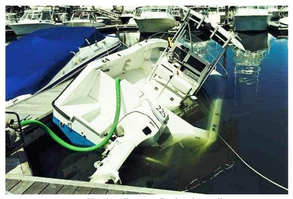
Note the well scuppers directly at the waterline. Note also the hatch mounted in the well that leaked, allowing water flow into the bilge, eventually sinking the boat.
