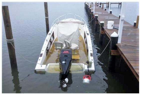
Repowering this older boat with a heavier four-stroke engine brought the scuppers and the waterline too low for the boat to survive a deluge.
