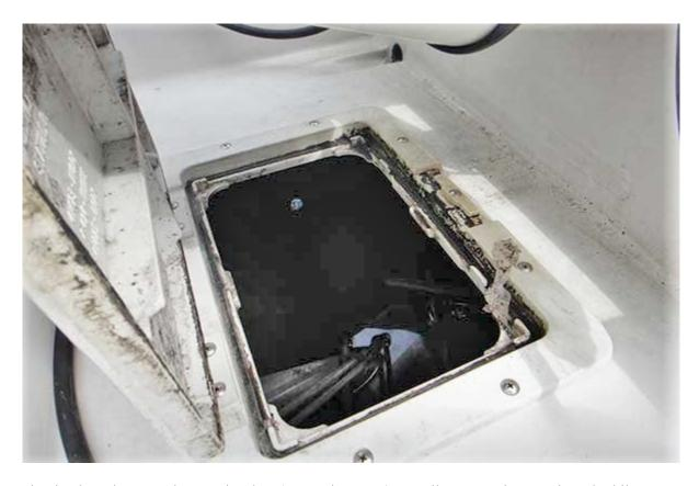
Poorly maintained or absent gaskets on hatches (even when new) can allow enough water into the bilge to overwhelm the pumps and sink the boat.
