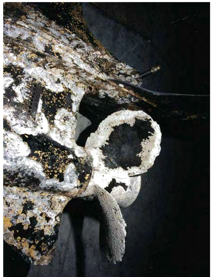
Stray current from a nearby boat overwhelmed the sacrificial anodes and destroyed this outdrive in a very short space of time. Source: BoatUS.
