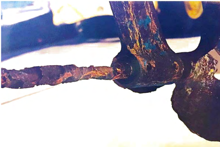
Stray current corrosion can damage underwater parts in a very short time. Wet slipped boats require regular testing of their surroundings for current flow entering their bonding systems.
